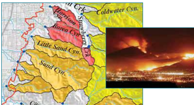
Figure 30—Probability of postfire debris flows associated with the Old Fire in Southern California. Red areas have highest potential, yellow areas the lowest. These risk models were developed by the U.S. Geological Survey and collaborators such as the U.S. Forest Service, Natural Resources Conservation Service, and various state agencies. Improved predictions of postfire effects are needed. Cooperative, interagency efforts offer the greatest potential for meeting critical information needs. Modified from Cannon et al. 2004.
