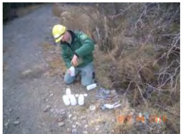
Below: Collecting water samples at the seep outlet with a hand pump (Left) and sample bottles (Right).
