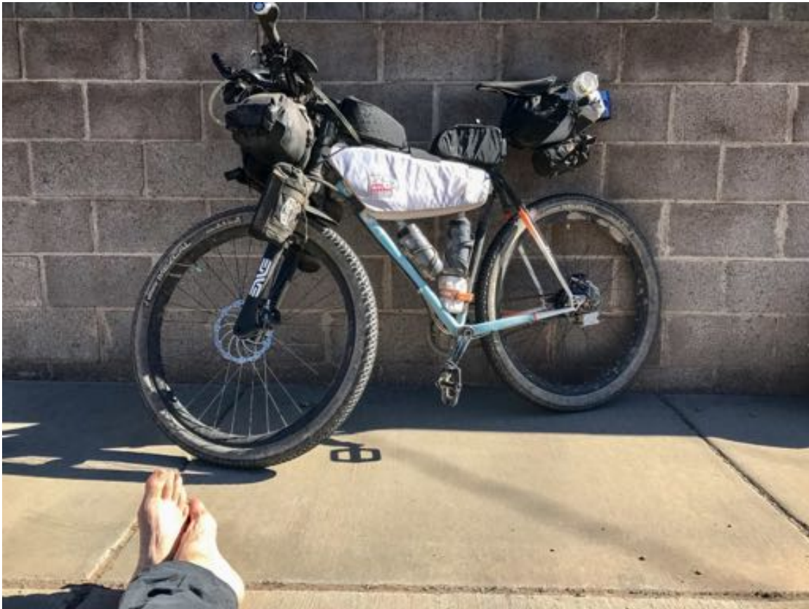
Figure 3: Example of a bikepacking bike. This bike was hand manufactured in Houston Texas, from the selection of tubing, geometry, and welding, by Matthew Schott, proprietor of Schott Cycles. It was ridden in the 2017 Tour Divide, a bikepacking event that spans 5 states and 20 national forests from Banff, Alberta Canada, to Mexico, along unsigned forest and jeep roads adjacent to the continental divide. The attached bike bags take the place of traditional touring racks and panniers.
