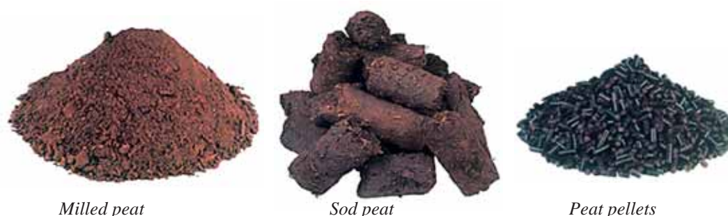
Figure 5.1. Different types of peat fuel. Source: Reprinted by permission of Vapo Oy.
