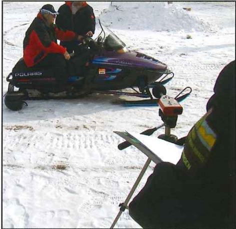
Photo by Kim Raap A snowmobile's sound level is being measured by a law enforcement officer using the SAE J2567 stationary sound test.
