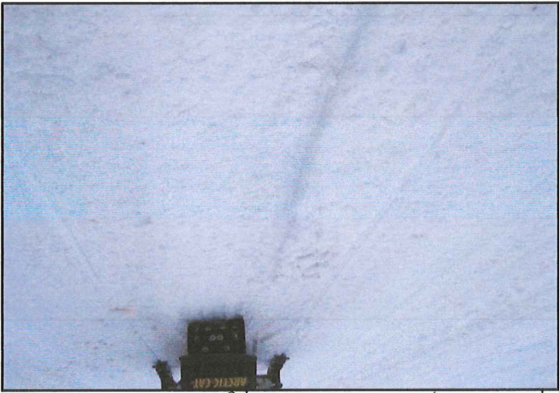
Photo 16: Snowmobile 1 (Arctic Cat Fire Cat 500) impressions from aggressive stop
